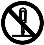
1. Do not remove the screw and do not open the cover if not said to do so in this User's Manual. If you ignore this warning, you may be burnt or receive an electrical shock due to a hot part or electrically charged part inside.
