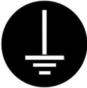
Ground the machine with a correct ground source or you may be electrically shocked.
