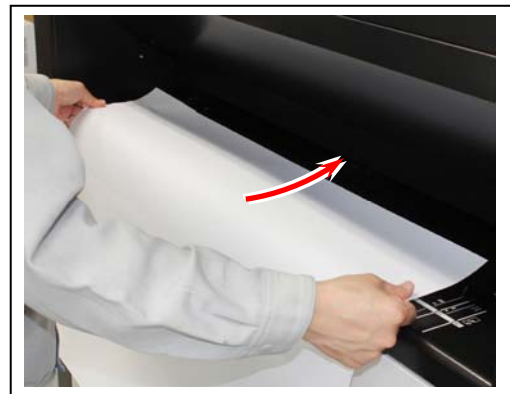
Incorrect (curl up)
