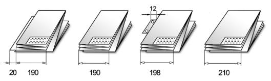
The package can be applied with a tab strip as shown in the third program. This is not part of the KIPFold 1000 functions and shown as an example only.
