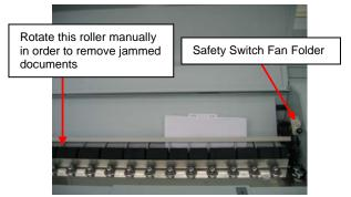
The folder will be powered off as a safety switch on the top cover cuts power at the same instance. As soon as you have lifted the cover, you will see the fan folder's inside. Retrieve documents stuck between the fold rollers by simply turning the fold rollers manually.
