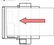
Insert the sheet <u>face down</u> (title block must be in front), aligning centrically. The insertion rail on the table can be slid into an optimized position for the document you are feeding. Please take care to feed the paper as straight as possible.
